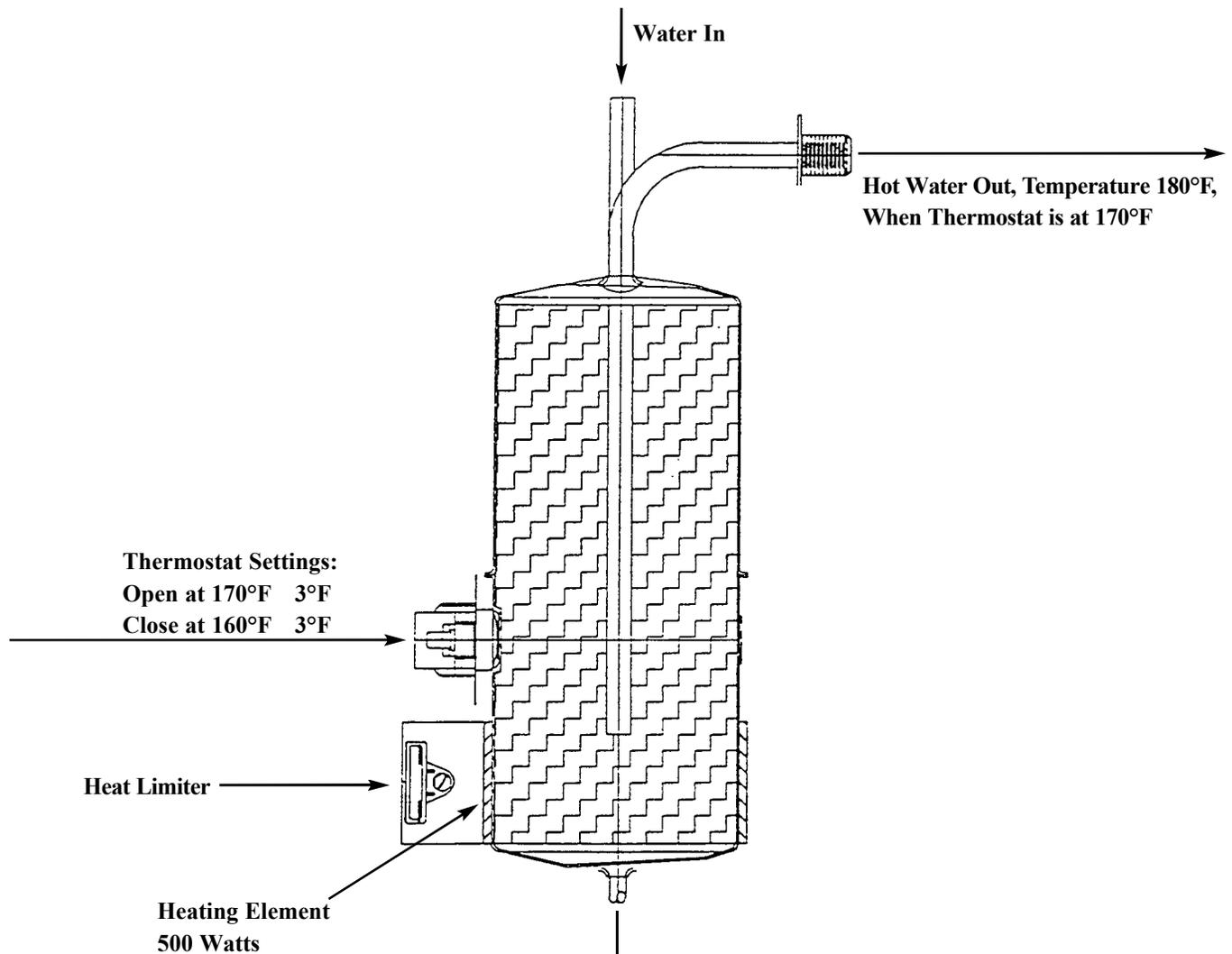
When water temperature at thermostat reaches 170°F, it opens up the circuit stopping power to the element. The temperature of the water at the outlet is 182°F. Now, if the unit is just left sitting without anyone using it, the water will cool to 160°F before the turning element turns back on again.
